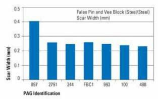
图表概况:基于ASTM D 3233, AISI 1137 steel 图表概况:基于ASTM D 2670, break block/AISI 3135 steel pin #10, break-in load 200 load @ 300 lbs for 60 minutes, lbs的故障负载(lbs), AISI 1137 steel block/AISI 313
